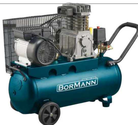
Air compressor belt driven • 4hp • 254Lt/min • 200Lt • 8Bar/115psi
