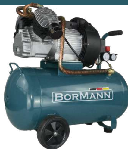
Air compressor direct driven, twin cylinder, oil lubricated • 3Hp • 336Lt/min • 100Lt • 8Bar/116Psi
